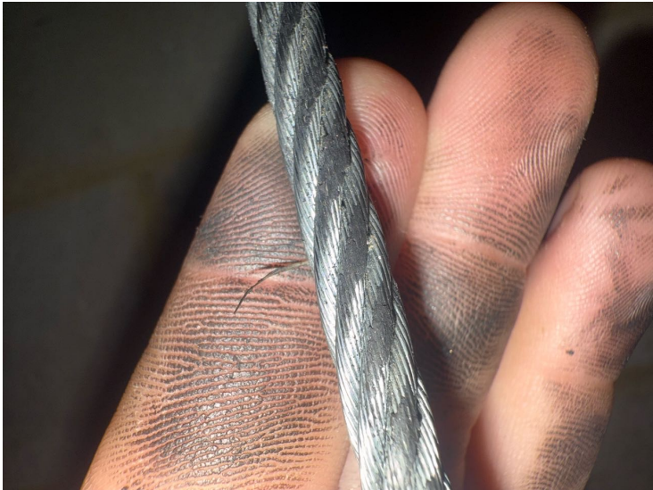
Safety rope is beginning to fray
